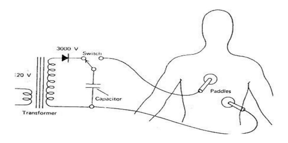
Fig. 4). A simple defibrillator. The line voltage is stepped up to several thousand volts by a transformer. A diode rectifies the alternating current into direct current to charge up the capacitor. When the switch is thrown. The capacitor discharge through the paddles and the heart.
