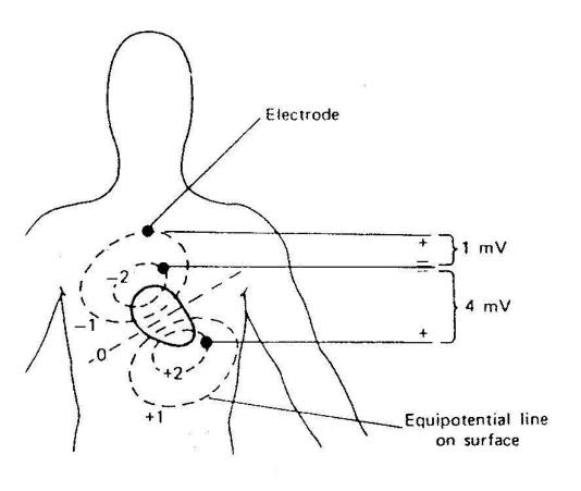
Fig.2. The dashed lines show the resulting surface potentials. The difference in the measured potentials caused by using different electrode locations. Both voltage and polarity my change with electrode position
