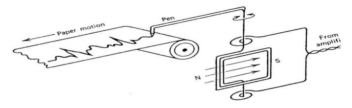
After amplification, the ECG signal must be displayed. When a routine diagnostic ECG is taken, a permanent record is required for analysis and a pen recorder is usually used (Fig.3). In a pen recorder, the amplifier output passes through a coil of wire suspended in a magnetic field. In the same way that a galvanometer twists when current passes through it, the pen twists to write on a moving strip of paper.
